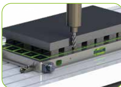
Turning and roughing the 2nd surface
