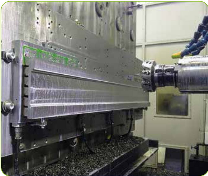
Milling of guideways, clamped in vertical tension on mobile pole extensions
